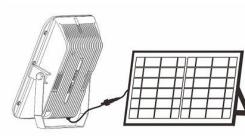
③Connect the lamp and solar panel with power cables.
